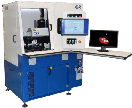
Engraving laser workstation - open
